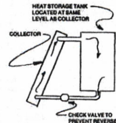
Fig. 7: A check valve prevents reverse flow when tank is even with collector.
